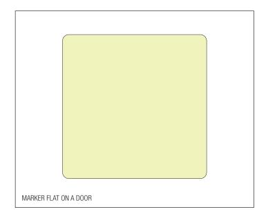
The Ecoglo "Door Handle Marker" is designed to ensure visibility of door handles in escape routes to meet NZBC Clause F6 "Visibility in Escape Routes". The door handle marker will be effective during failure of the main lighting.
