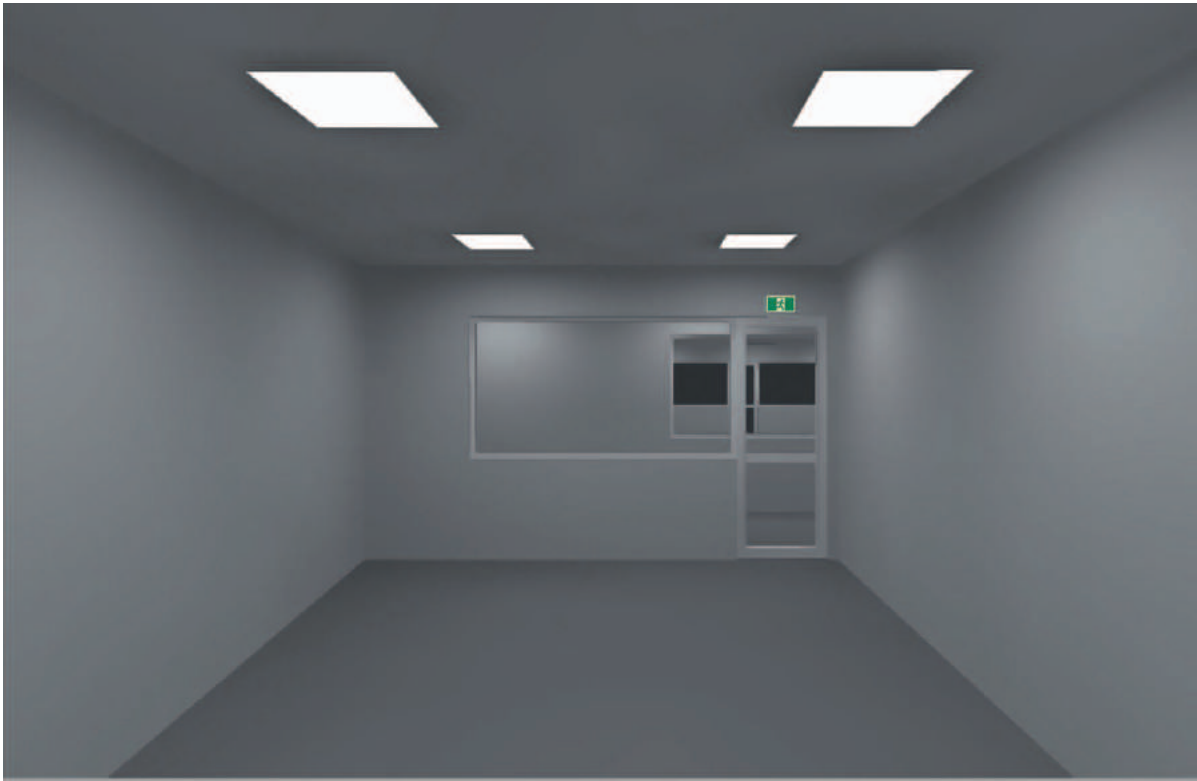
View 3. 214 lux illuminance on the sign from electric lighting.
