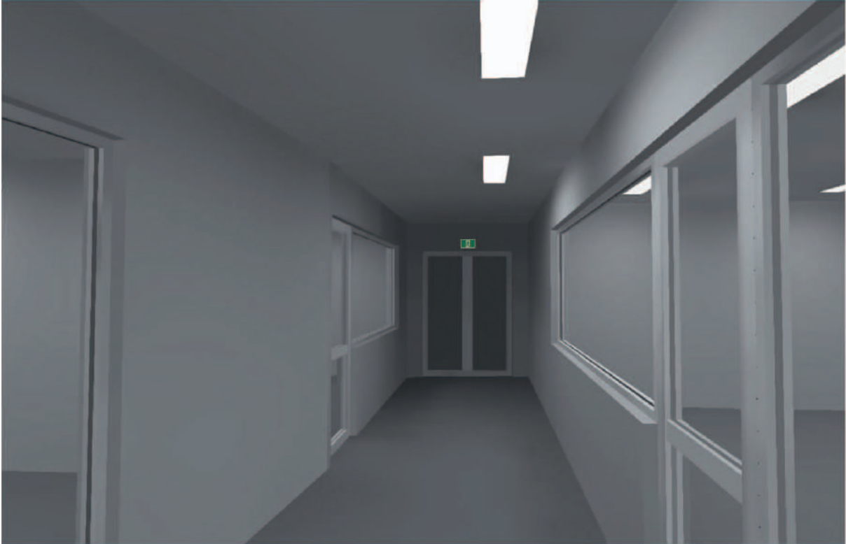
View 7. 50 lux illuminance on the sign from electric lighting. Insufficient lighting scenario.
