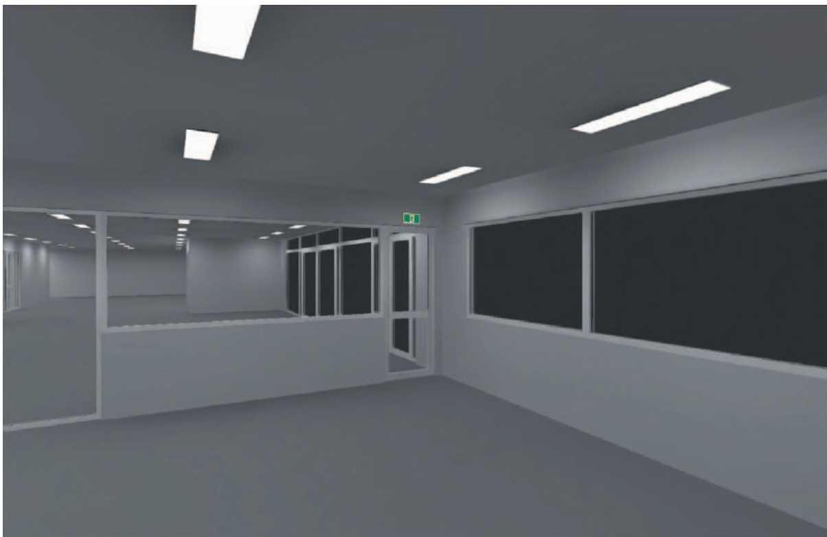
View 2. 136 lux illuminance on the sign from electric lighting.
