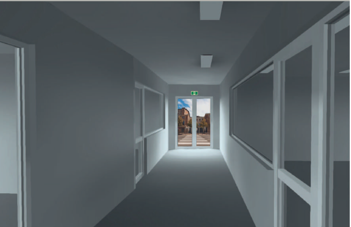
View 6. 20 lux illuminance on the sign for a min. of 6 hours per day from natural light.
