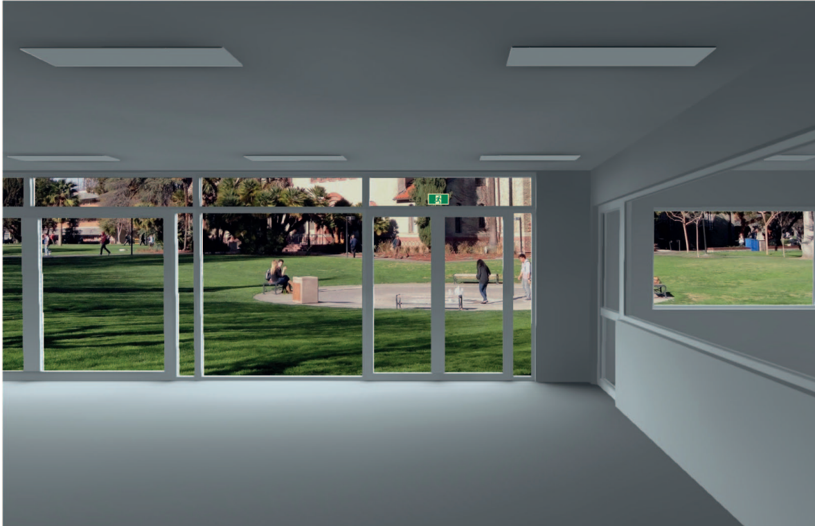
View 1. 65 lux illuminance on the sign for a min. of 6 hours per day from natural light.
