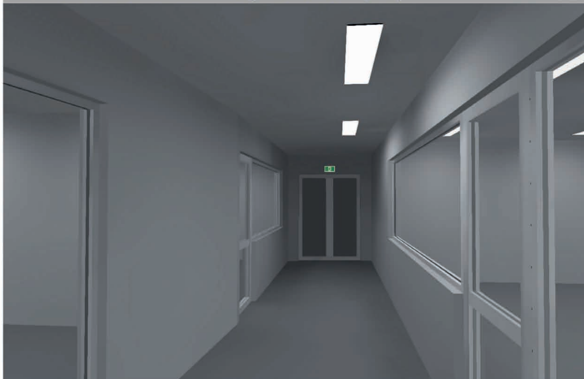
View 6. 65 lux illuminance on the sign from electric lighting.
