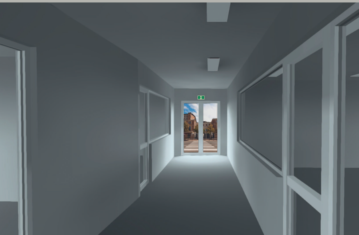
View 6. 20 lux illuminance on the sign for a min. of 6 hours per day from natural light.
