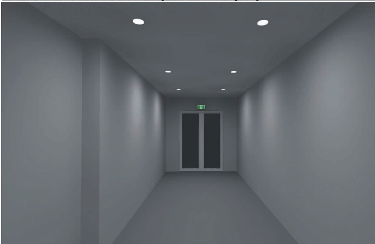
View 4. 98 lux illuminance on the sign from electric lighting.
