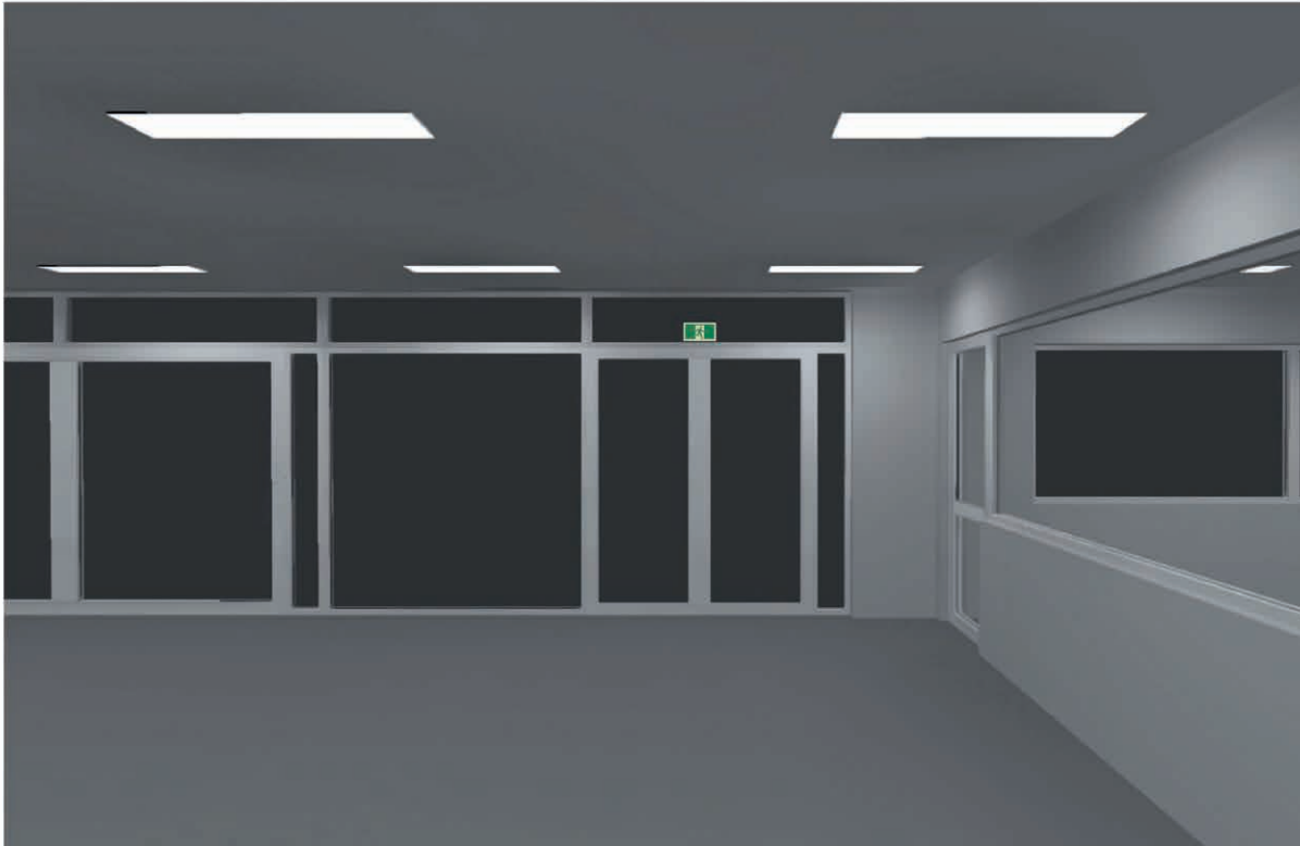
View 1. 167 lux illuminance on the sign from electric lighting.
