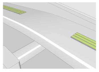
Do not bend guidance strips over bends. Set the strip 50mm from the bend.
