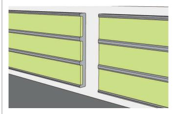
Where strips are to be butted together, there must always be a 3mm expansion gap between them. This allows for expansion and contraction between the Ecoglo strip and the building surface.
