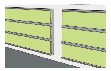
Where strips are to be butted together, there must always be a 3mm expansion gap between them. This allows for expansion and contraction between the Ecoglo strip and the building surface.
